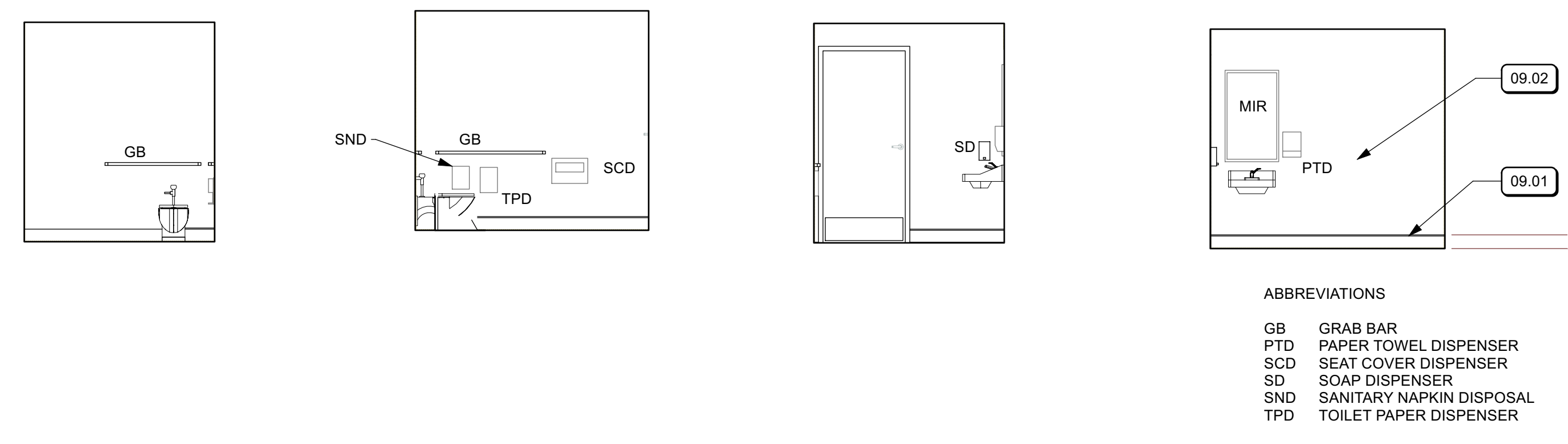
4 TOILET ROOM TYPICAL ELEVATIONS Scale: 1/4" = 1'-0"
